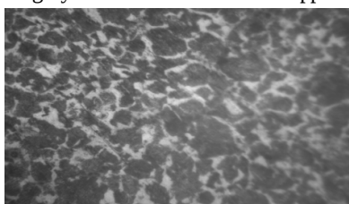
Plate 1: Microstructure of 25 mm Diameter of Rolled Ribbed Medium Carbon Steel. (X400) Etching time: 3 seconds and Etchant: 2% Nital
